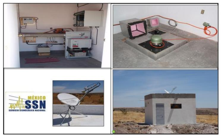
The core for the National Broadband Seismic Network is composed with stations equiped with Quanterra dataloggers, seismometers STS-2, and accelerometers Episensor ES-T. For real time transmission at rural areas, the SSN uses a VSAT station.
